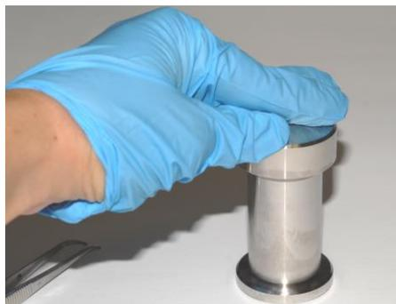
After inserting the sample, insert the plunger and press down on it with the hand to compress the sample, driving out any ambient air (i.e. nitrogen) and forming the pellet.
