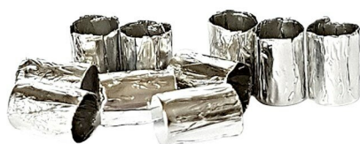
Tin capsules pressed standard weight 5 x 3.5mm
